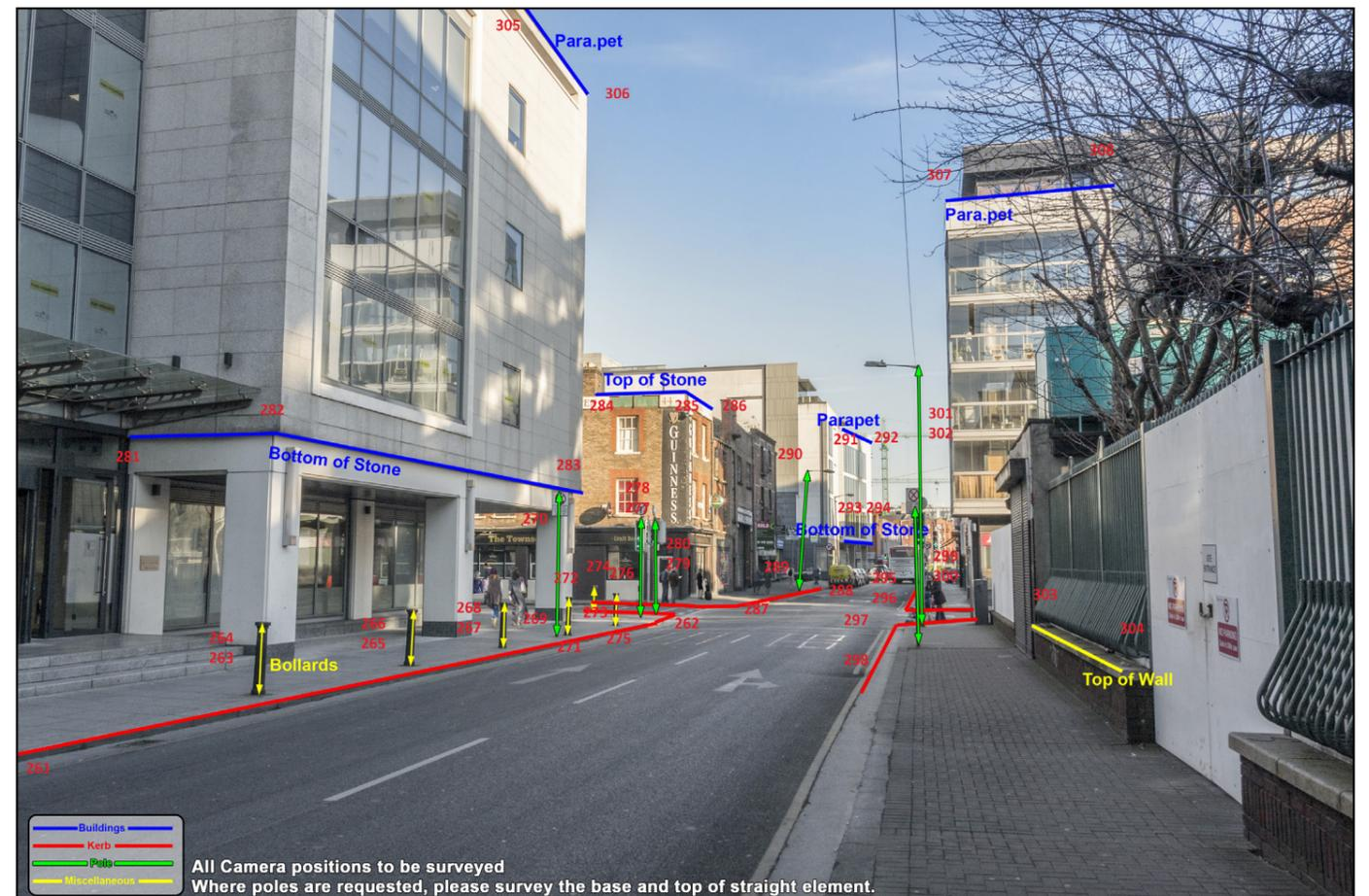
Fig.8: Fixed reference points fully surveyed and numbered.
